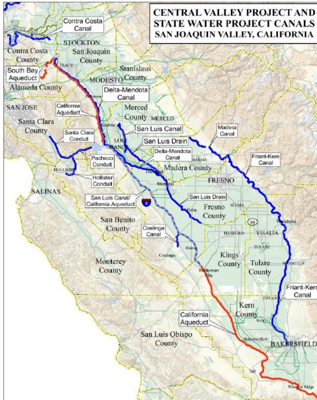
Central Valley Project and State Water project canal system Blue line: Federal (CVP) Red line: State (SWP) Green line: Private Blue/Red line: Joint Federal/State Scale: 1:1,500,000
